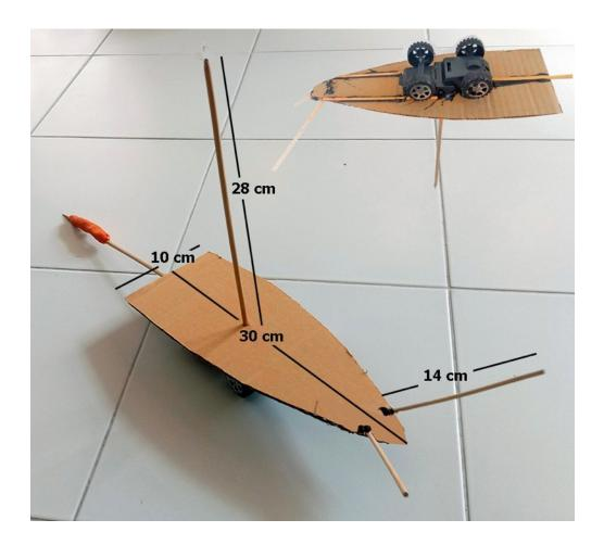
The model has wheels, deck, mast, ballast beam and three attachment points for a sail. The sail is really important. The contraption must go in a straight line in a gusty wind so it must self-correct without anyone steering.
