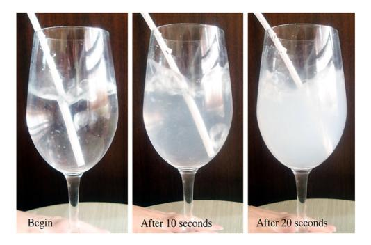
Lime water turns "milky" as calcium hydroxide,  $Ca(OH)_2$ , is converted to limestone powder,  $CaCO_3$ .
