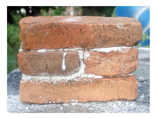
The mortar has hardened as expected but it has not stuck to the bricks. The wall can be taken apart. *We will have to think about that.*
