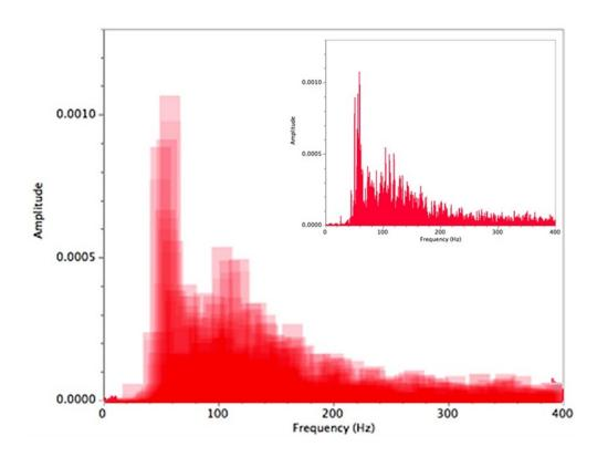
The original high resolution sound spectrum (inset) has been blurred to show the structure in lower resolution. There are two resonance peaks: one at  $\sim$ 55 Hz and a lower amplitude broader peak at  $\sim$ 110 Hz.
