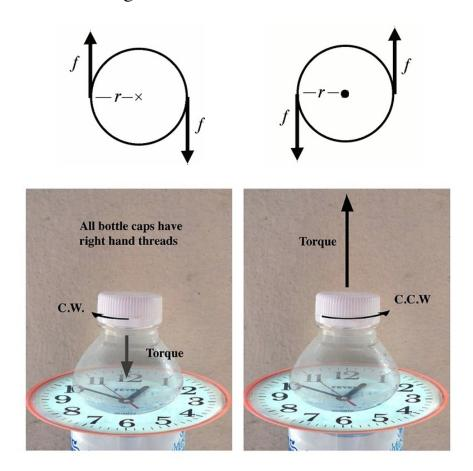
The cap is tightened by turning it clockwise (left).
