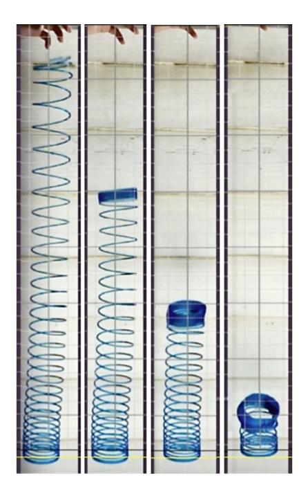
Four frames from the video, at equal time intervals, show that the top rings fall at almost constant velocity as the lower turns remain almost stationary.
