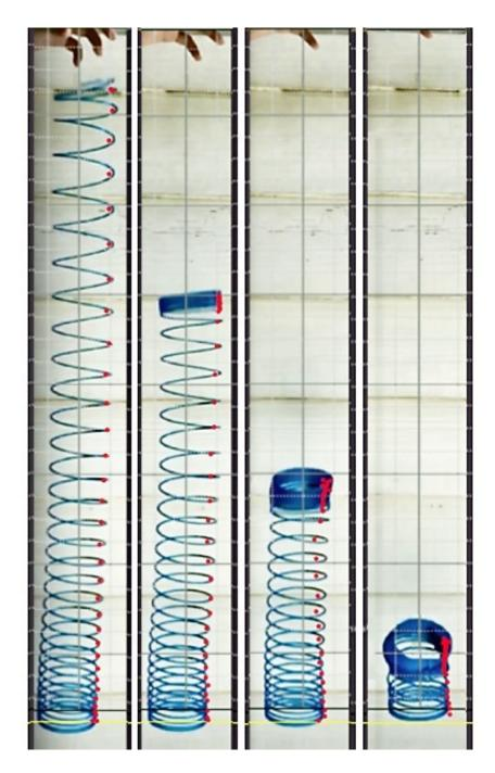
Because the lower rings are stationary (the same in each frame) data from column 1 *could* be pasted to later columns, but a mistake would then be propagated through all columns. For that reason a line of dots marking turn positions was put on each frame independently, making sure each data table had 34 data entries.
