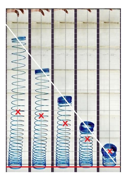
The unexpected feature of this illustration is the slight lifting of the lowest turns before the spring completely collapses. This *second order effect* may be associated with the forward rotation of the upper coils on the right, possibly because the spring is not completely uniform, or the descent may be influenced by increased air resistance between the spring and the wall.
