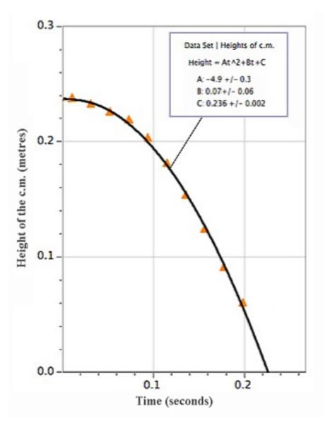
The position of the c.m. as a function of time in seconds.
