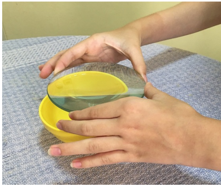
A large magnifying glass (biconvex lens).
