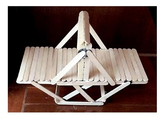
The deck is 8 cm wide and rests on the two girders. Cross ties have been added above and below to keep the side frames in line as weight is added to the deck.
