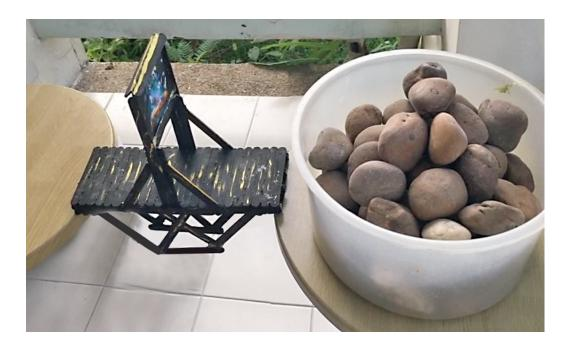
The bridge was placed between two chairs. The pot of 100 gram stones had a measured mass of 5.4 kg. A bag was hung on the bridge as shown below and stones were added one at a time.
