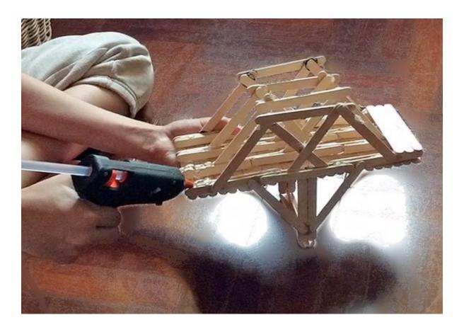
The two new frames were fixed with hot glue to the decking and additional decking was added at both ends to provide a firm support at the sides of the 20 cm gap.
