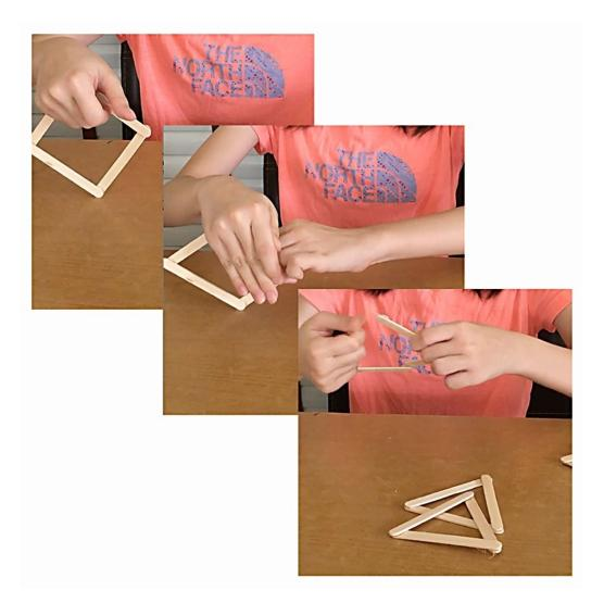
The squares could be dismantled quickly and easily by pushing them out of shape to wrench and weaken the glue but to my surprise the triangles couldn't be taken apart without breaking the sticks. Given that: and the challenge we were given: to make a bridge with a hundred or so popsicle sticks that looks pretty, spans a 20 cm gap and holds five kilograms, we designed a bridge that looked a bit like the two examples below.
