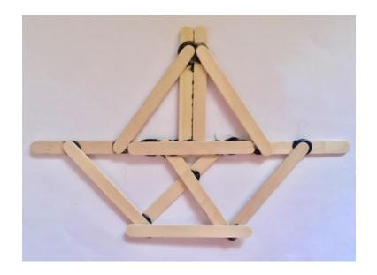
The frame is made with 9 cm popsicle sticks. It has a laminated horizontal girder 22 cm in length with two triangles on top and four below. We made two of these: one on each side of the decking.
