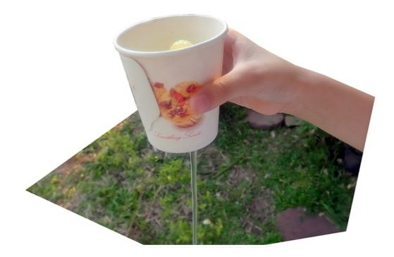
The water flow is driven by the small difference in pressure between the lower end of the siphon in the cup and the lower end outside.
