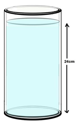
The pressure at the bottom of the water is given by  $\rho gh$  as before.
