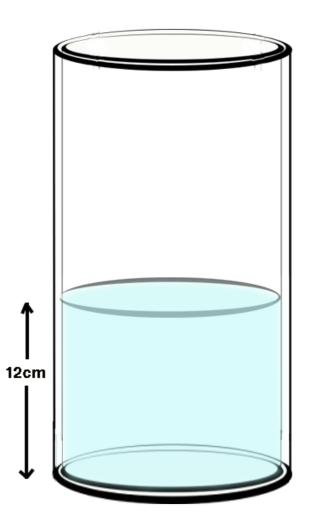
A weight of 12 cm of water pushes down on the base, of area A.
