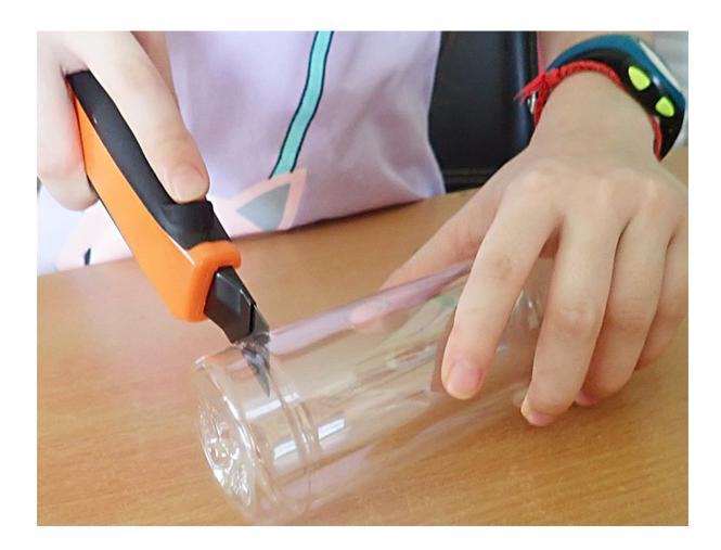
The curved side of the bottle was flattened out and strips were cut at an angle of 45° to the vertical. A pot of water was boiled. The water temperature was found as it cooled with an alcoholin-glass thermometer, being careful to stir the water to make sure the temperature was the same everywhere.
