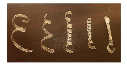
The plastic went into tighter spirals at higher temperatures. Coil diameter in mm versus water temperature is plotted below.
