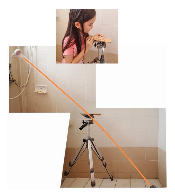
**1** I made the shower hot. Close to the shower-head the water was 44.0 °C. At one metre (half way to the floor) it was 41.0 °C. At two metres (just above the floor) it was 38.0 °C.
