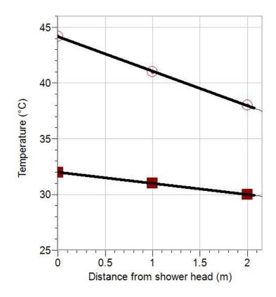
The line graphs are both straight. When the shower is hot the temperature drops three degrees per meter. When it's cooler the temperature drops only one degree per metre. The temperatures are less different but the same thing happens. The water cools towards the floor.
