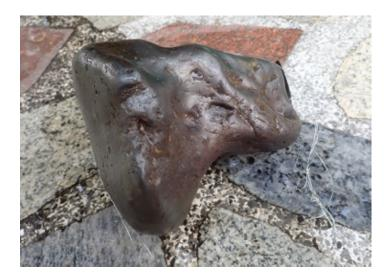
To find the volume of the rock it was hung on the scales in a bucket of water. That sounds silly, but it's clever.
