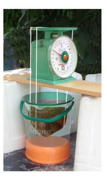
The loss of weight under water is 1110 g, meaning that the mass of water with the volume of the rock is 1110 g. The density of water is 1g/cc.
