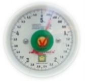
When the rock is under water the balance reads 4180 g.
