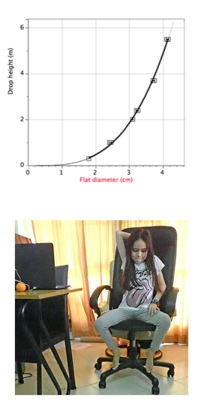
I sat in a chair and hurled the ball at the floor. The diameter of the flat bottom when I threw the ball (4.3 cm) was the same as it would have been if I'd dropped it from a height of 6 metres.
