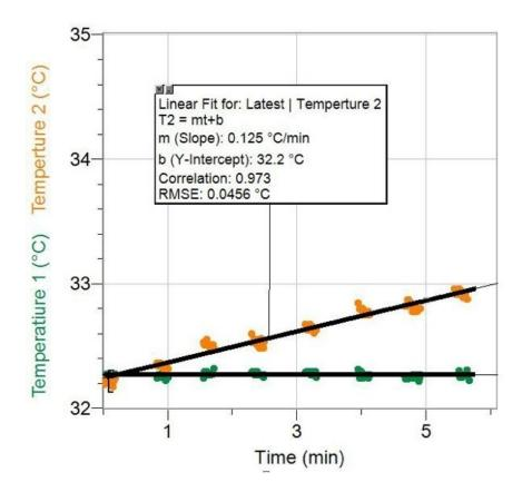
After each set of ten drops the temperature of the deformed clay rose by a small amount. The small scatter of points shows the accuracy of the temperature measurements. The orange data plot is a straight line with a slope of 0.125 °C/min. Ten drops raised the temperature by the same amount each time.
