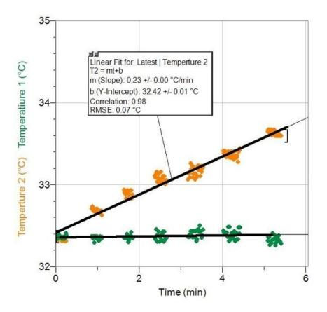
This time the ball temperature rise was less on the clay pad than when it had hit the floor.
