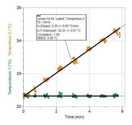
Effectively dropping the ball from three times the height (6 m) increased the temperature rise by about three times.
