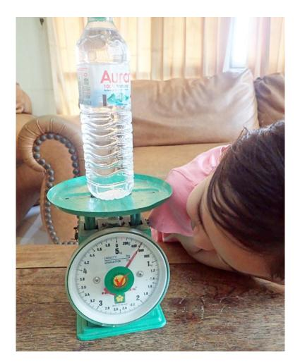
**1** The measured mass of the half litre bottle of water was close to 500 grams. The balance was reading correctly. The density of water is 1g/cc.
