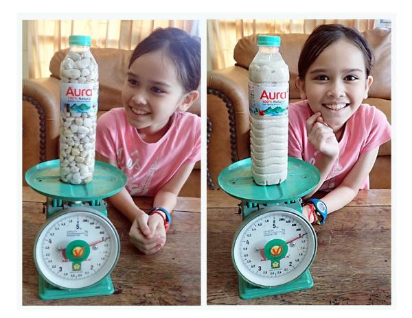
The mass of each bottle topped up with water was 1000 g = (800+200) g. The same amount of water (200 cc) was added to each bottle. The total empty space between the stones and the sand was the same in each case (200 cc) and the volume of the rock (quartzite) was 500-200 = 300 cc.
