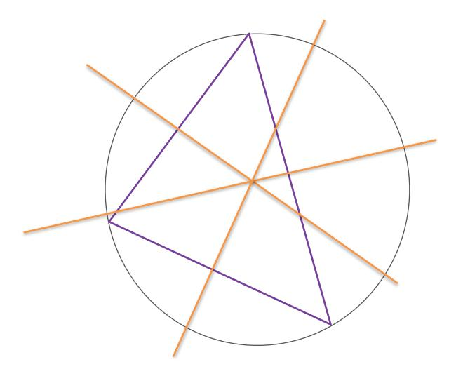
Perpendicular bisectors of the sides of a triangle intersect at the centre of the *circumcircle*, passing through all three vertices (points). Find the equal line segments and the right angles on the diagram.
